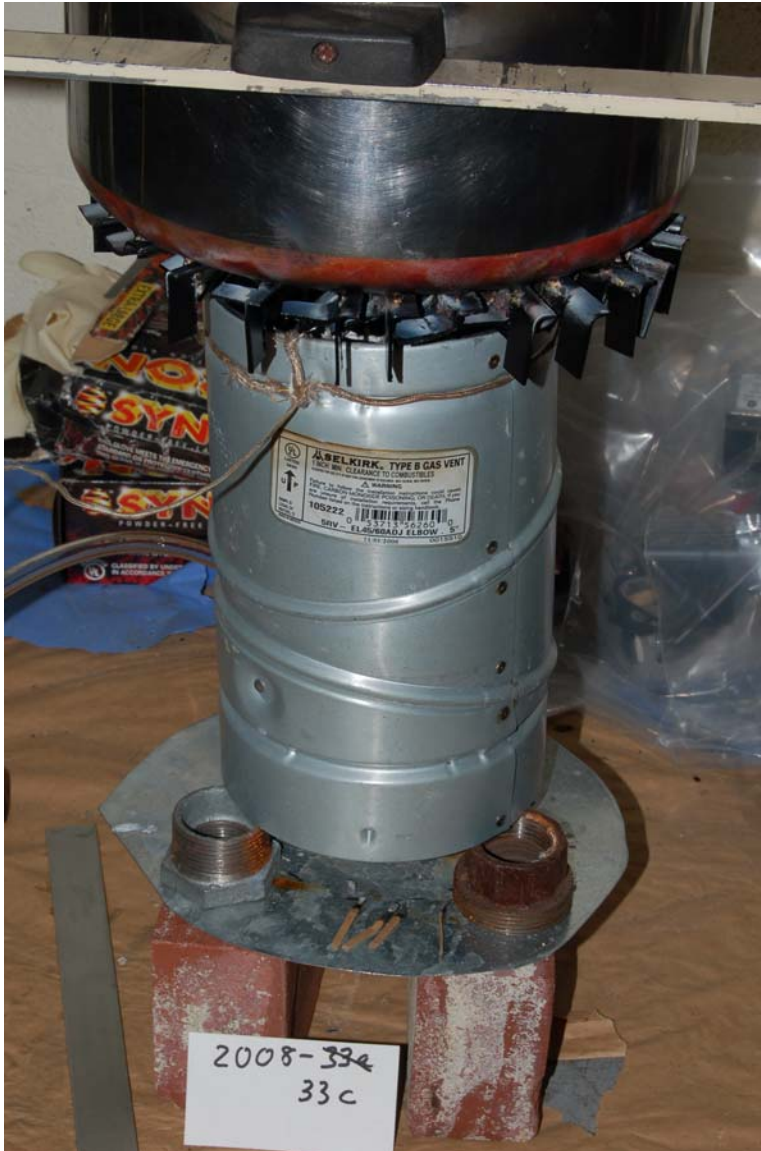
Figure 2: Simulated rocket stove.
