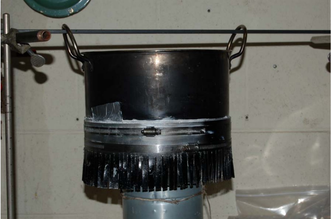
Fig. 9: Overall view of the slit fin pot being tested on the simulated rocket stove. Note that the standard pot was used.
