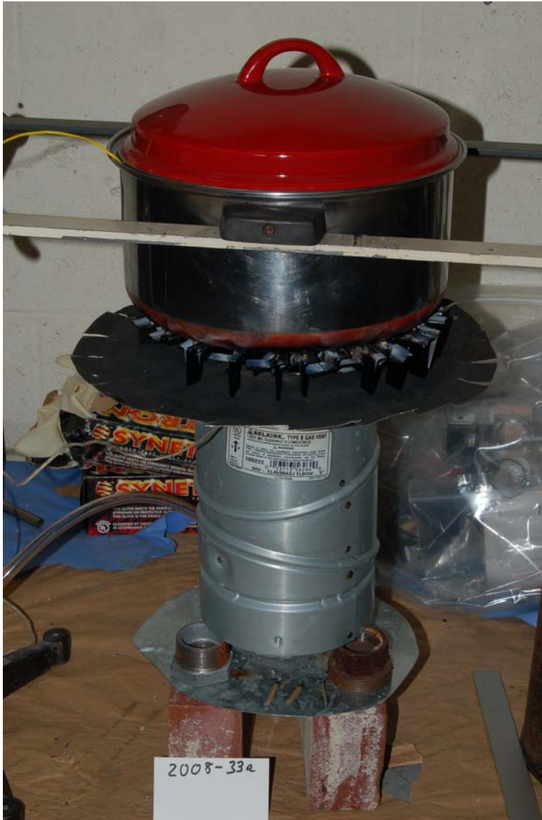
Fig. 3 The simulated rocket stove with base.
