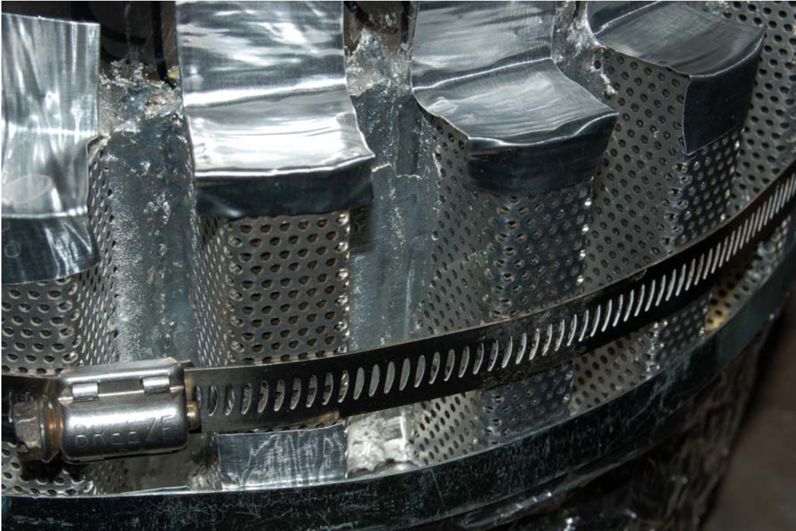
Fig. 9: A portion of the standard-size pot with perforated metal fins. The channels through the fins are blocked at the top, as shown.
