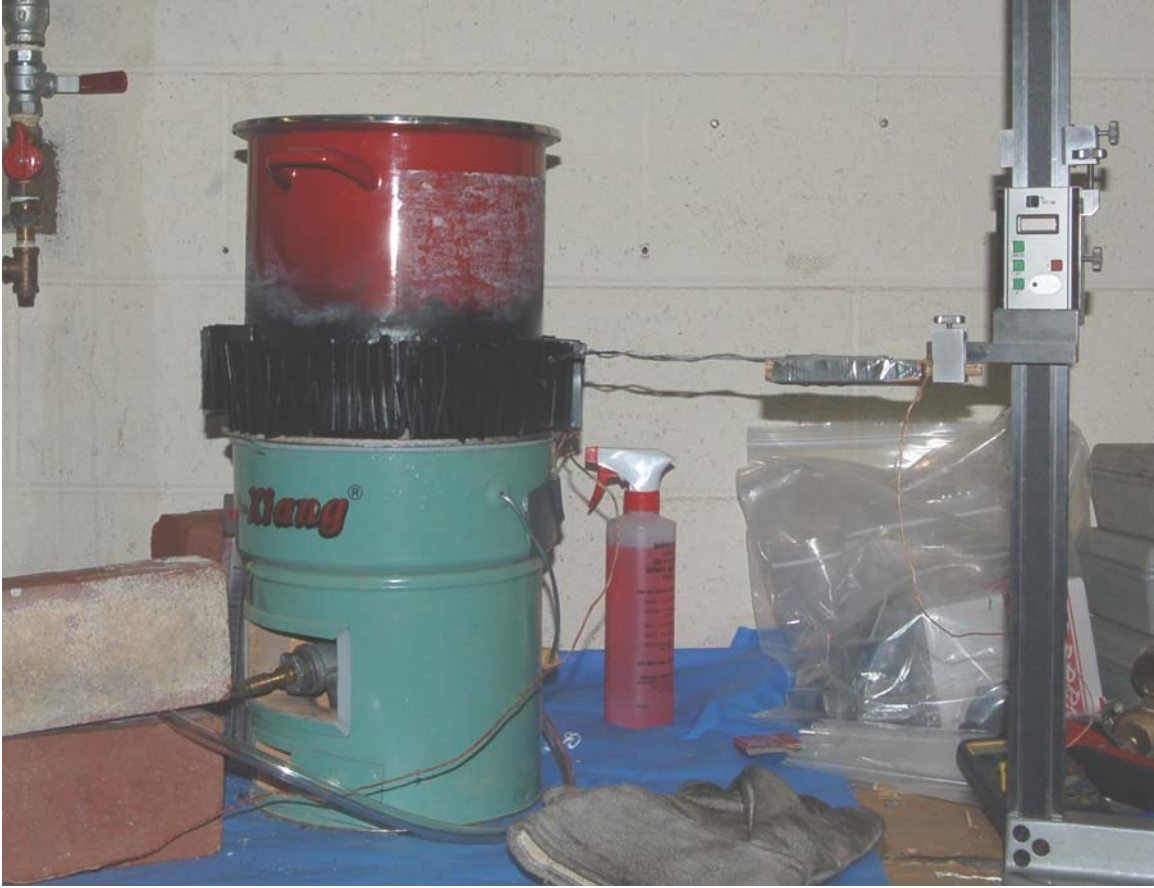
Fig. 4 The Chinese rocket stove, modified to run on natural gas.
