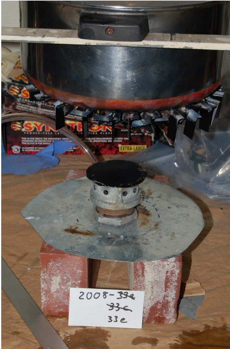
Figure 1: The simulated open fire.
