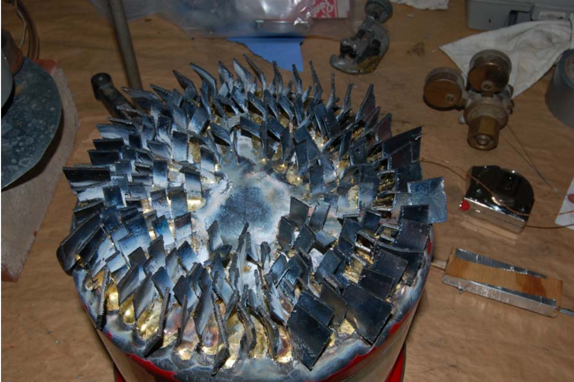
Fig. 5: The final design of the bottom-finned pot.
