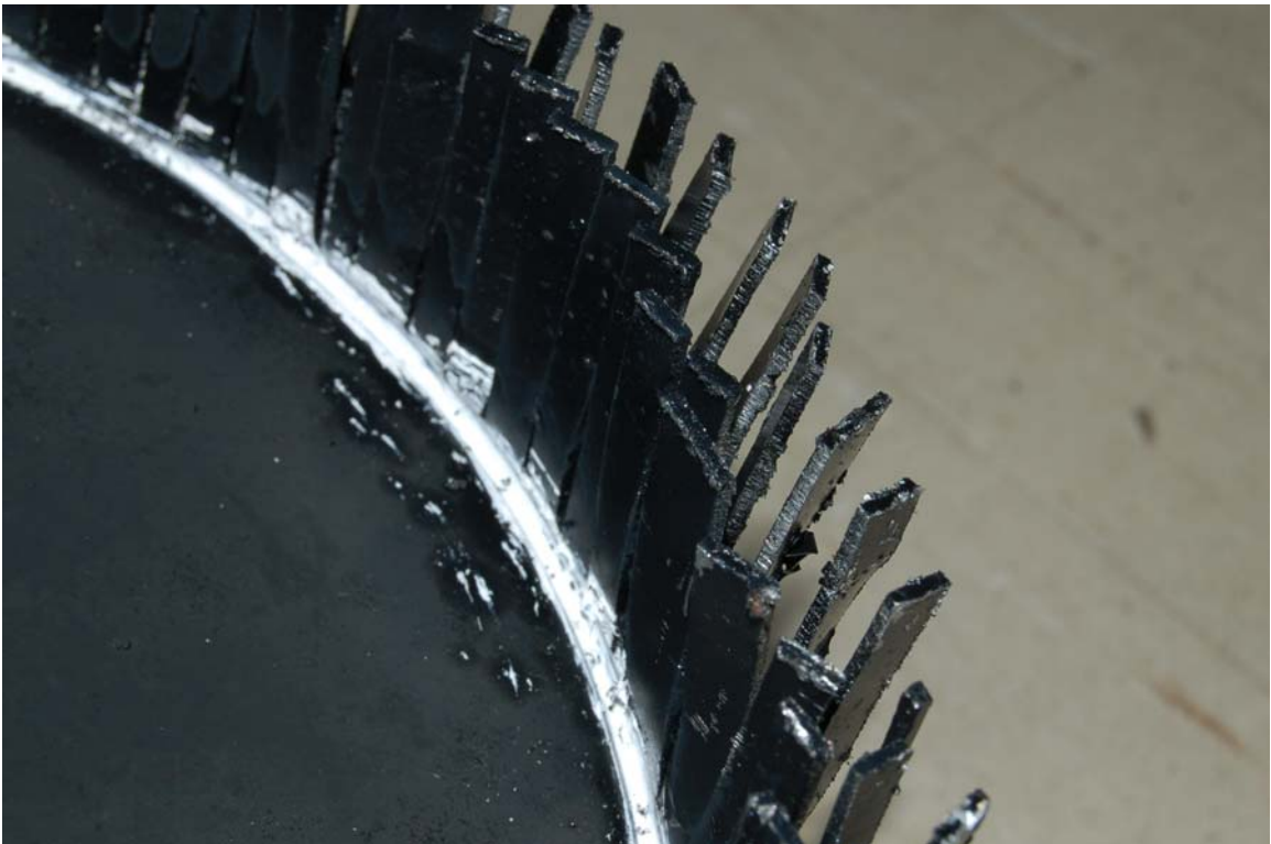
Fig. 10: Close up of the slit fins.
