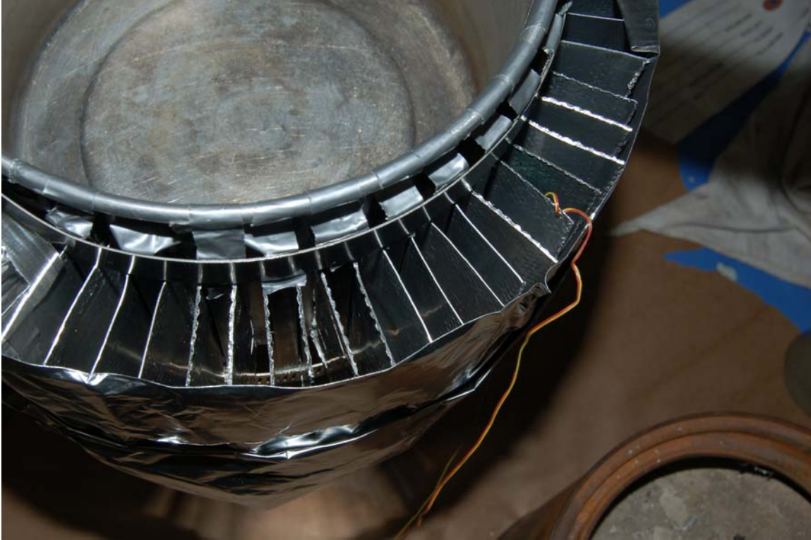
Fig. 7: Close up of the top of the fins. This was one style of fins that was used, other styles were also tested.
