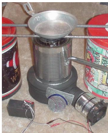
Fig. 2: Shown is a Juntos B+ TLUD with forced air. (Source: Anderson and Reed LAMNET article in 2004.)
