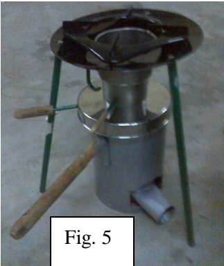
Lid of 5-gallon bucket, plus legs and coupler.
