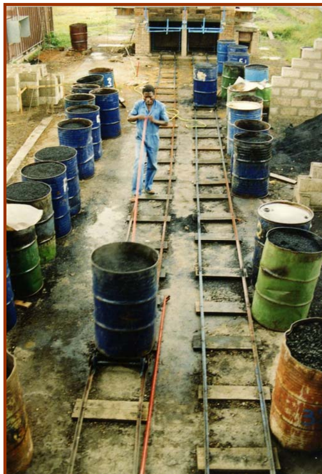
Photo 5: rails for moving containers filled with charred biomass (charcoal) from the CCS
