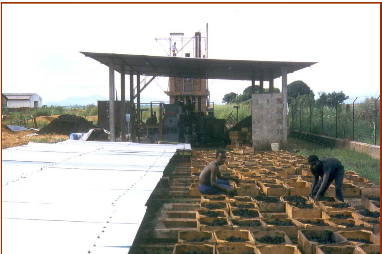
Photo 1: moveable hangars (rain protection) for solar drying of the bio coal briquettes
