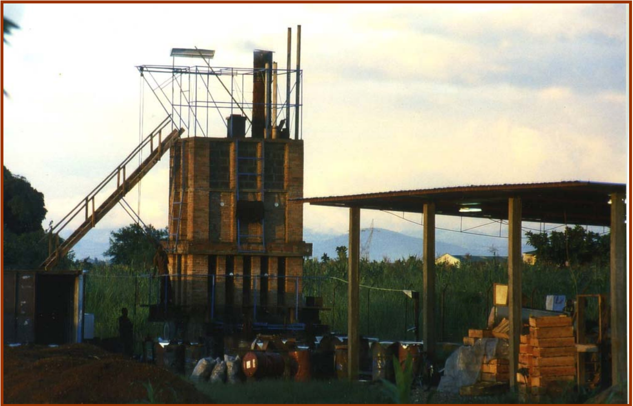
Photo 4: close up of the Continuous Carbonization System (height without chimney: 6.5m)
