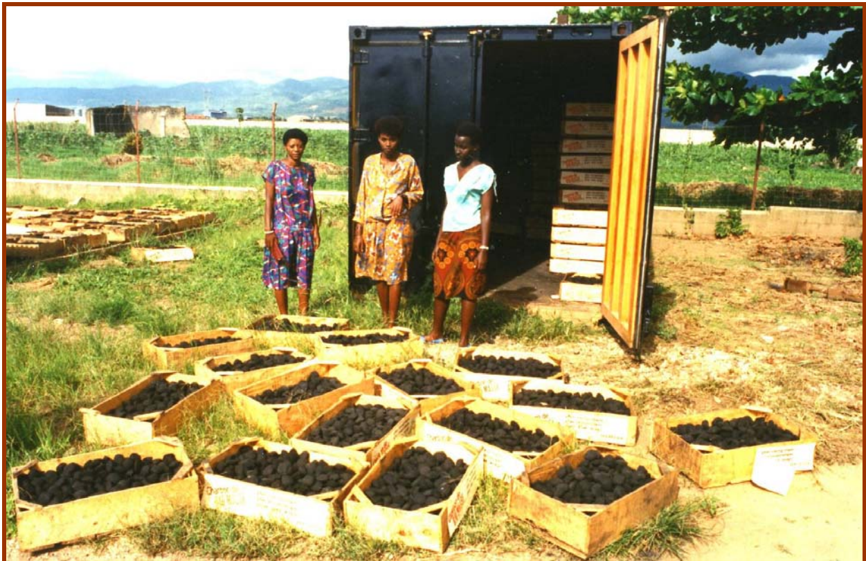
Photo 3: storage room for bio coal in a solar heated container (black coating)
