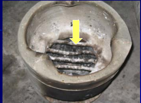
The traditional charcoal stove made of cement with iron bars as charcoal holder.
