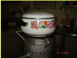
Rice Husk Gas stove made by a local artisans under the guidance of IDEA staff member
