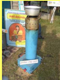
Rice Husk Gas stove made by a factory under the guidance of IDEA staff member
