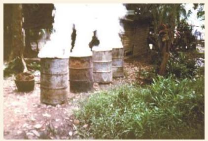
Vertical drum kilns were used for coconut charcoal making
