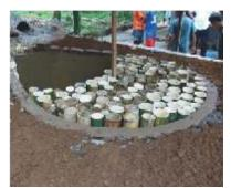
Bamboo stew are arranging into the Iwate kiln
