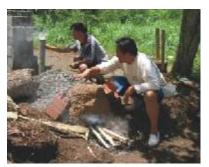
Adjusting the air flow at the mouth of horizontal drum kiln
