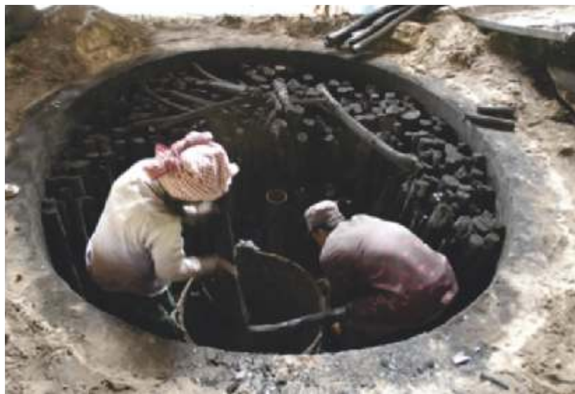
Arranging the wood into the Yoshimura kiln
