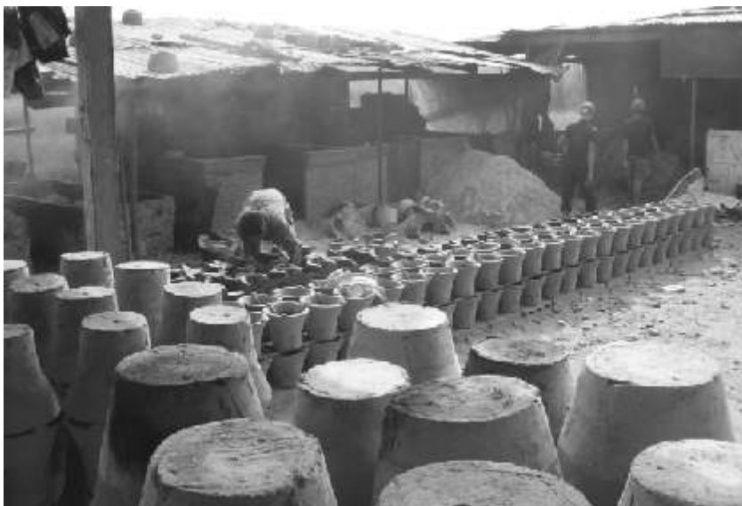
Sun-drying the stoves before firing in the kiln
