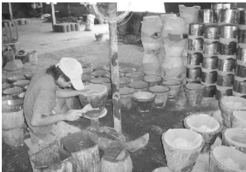
Making the stove body using a mold
