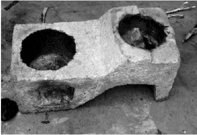
Econo-Dalikan, concrete ICS, developed at Appropriate Technology Center, Central Philippines University
