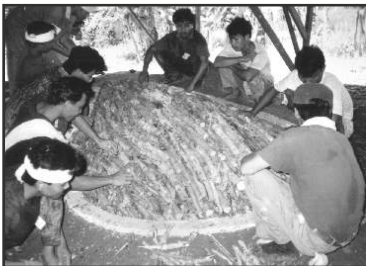
Figure 2 Arranging the wood in the kiln before ignition
