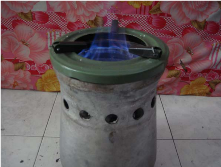
Figure 4: Small gas cooker (for household with 1-3 persons) generates gas “ Vietnam Magic Fire ” with Pellet BioCarbon coal based fuel burnt to become gas, which is invented by Prof. Tran Binh.
