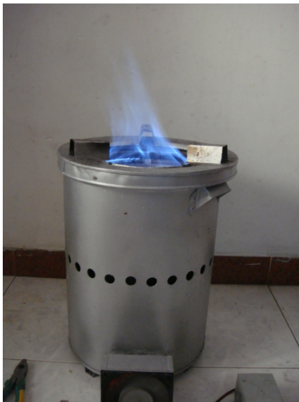
Figure 5: Medium gas cooker (for household with 4-6 persons) generates gas “ Vietnam Magic Fire ” with Pellet BioCarbon coal based fuel burnt to become gas, which is invented by Prof. Tran Binh.
