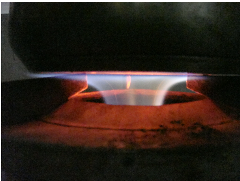
Figure 6: Medium gas cooker (for household with 4-6 persons) generates gas “ Vietnam Magic Fire ” with Pellet BioCarbon coal based fuel or Shaped Biomass burnt to become gas, which is invented by Prof. Tran Binh.
