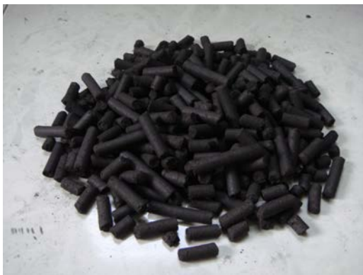
Figure 1: Pellet BioCarbon coal based fuel is burnt to become gas, which is invented by Prof. Tran Binh.
