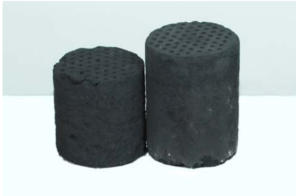
Figure 2: Shaped Biomass coal fuel, which is invented by Prof. Tran Binh.
