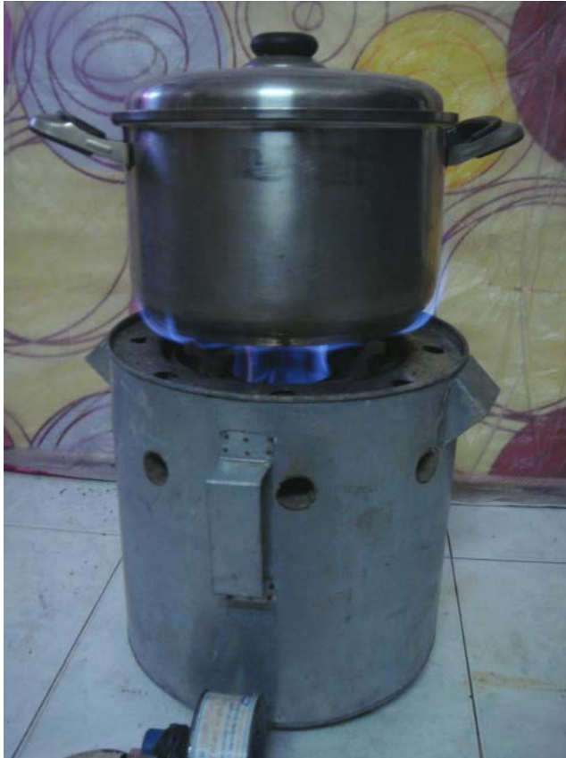
Figure 6: Medium gas cooker (for household with 4-6 persons) generates gas “ Vietnam Magic Fire ” with Pellet BioCarbon coal based fuel or Shaped Biomass burnt to become gas, which is invented by Prof. Tran Binh.
