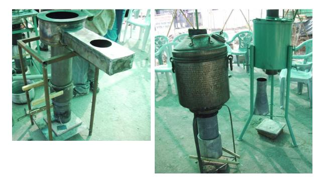
TLUD stoves made in India. Note the sliding connectors. Several are for water heating.
