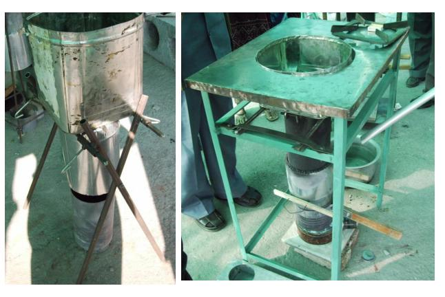
The "X" legs hold the horizontal bars that hold the stove's upper body.
