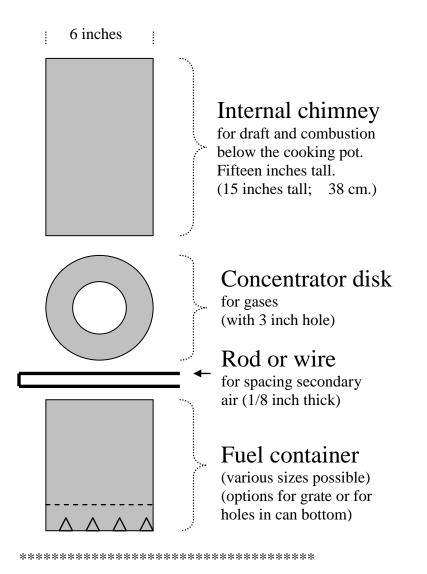
The 1/8<sup>th</sup> inch diameter spacer rod is to be 1) under the horizontal concentrator disk, and 2) on top of the upper lip of the fuel container. This gap has proven to be correct for the Champion 6-15 stove as tested thus far. The two arms of the rod or wire should be parallel and separated slightly more than the 3 inch diameter of the hole in the concentrator disk. The use of one rod that is bent into a "U" shape is convenient, but two separate rods would work equally well.
