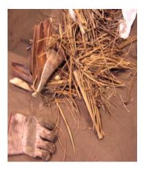
Pieces of coconut fronds (leaves) that can be combusted in a TLUD gasifier. The pieces should be smaller than these. Maximum 2 inch lengths.
