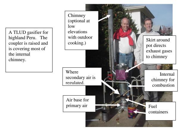
b. Support from below is typically like stacking two boxes or cans on top of each other, with the upper one holding the pot on top and the internal chimney inside, while the bottom one has one side cut open to allow the placement and changing of the fuel container.
