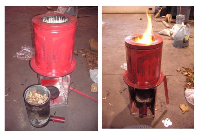
The disk in the bottom rises under the fuel canister, and is held in the raised position by the red stick on the outside. Note the metal controller of the primary flow.
