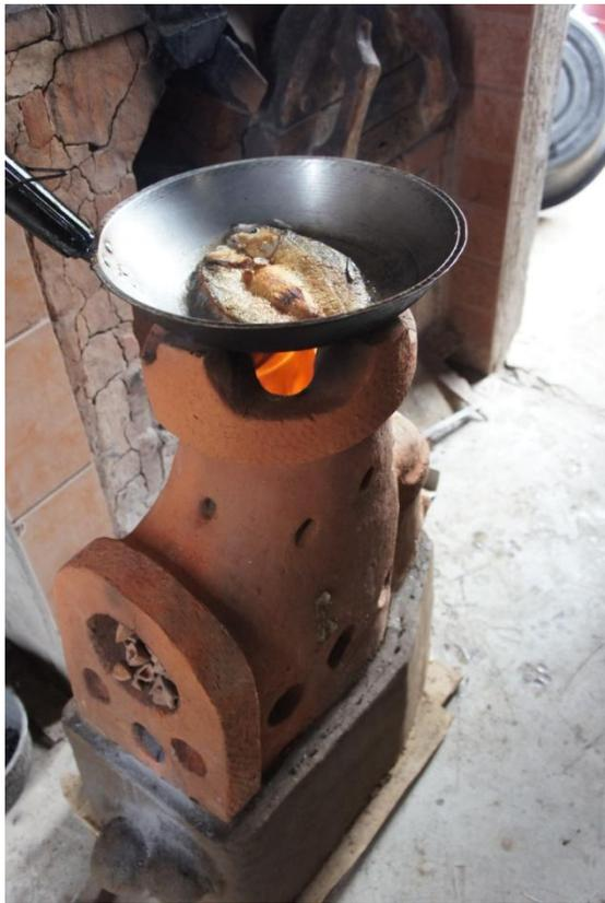
AND MORE WERE PUSHED INTO THE FUEL SHELF WITH THE HELP OF THE PUSHER ROD. THIS LEAVES A NEW SPACE WHICH ALLOWS MORE FUEL TO COME IN.
