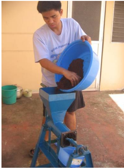
Loading of Mixture of Cocopeat and Gelatinized Starch in the Machine
