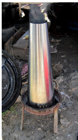
Figure 1 – Lighting cone on a traditional Haitian stove.
