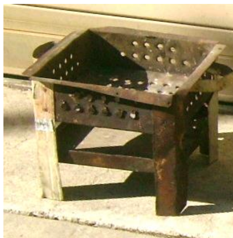
Figure 2 – Traditional Haitian charcoal stove used for testing.
