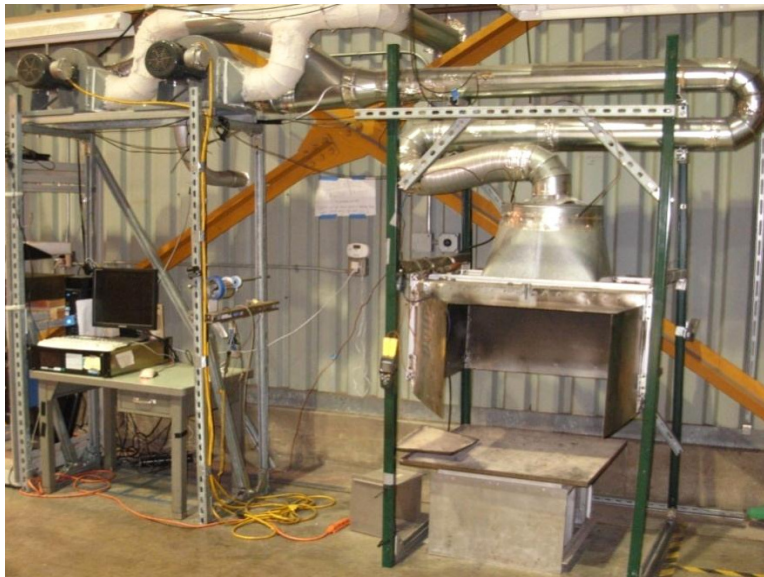
Figure 3 – The stove testing system at LBNL. The exhaust hood and ductwork are seen on the right-hand portion of the photo; the instrumentation is on the left.
