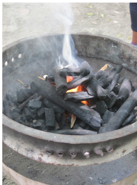
Figure 7 – Fully stacked charcoal bed.
