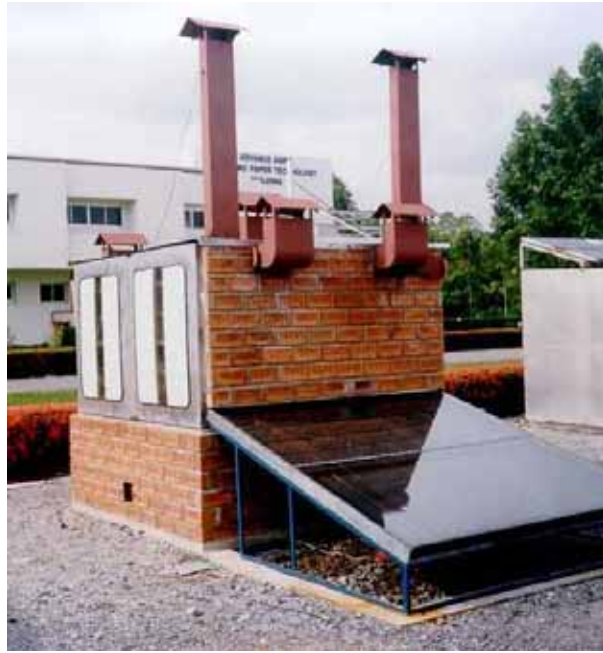
Figure 2.2 Solar-biomass hybrid cabinet dryer
