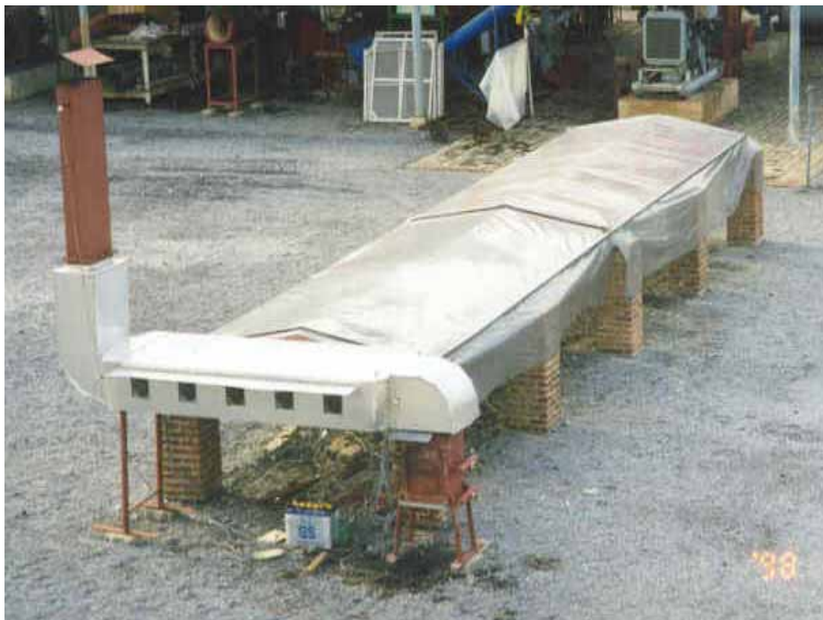
Figure 3.1: The solar-biomass hybrid tunnel dryer
