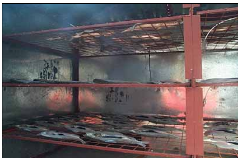
Figure 10.3: Drying chamber of the hybrid dryer
