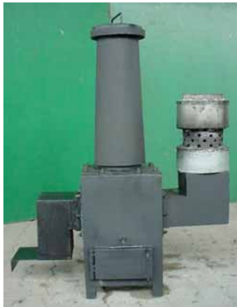
Figure 2.5: Fully assembled domestic gasifier stove
