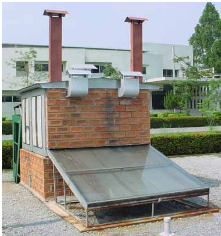
Figure 2.20: The solar-biomass hybrid cabinet dryer
