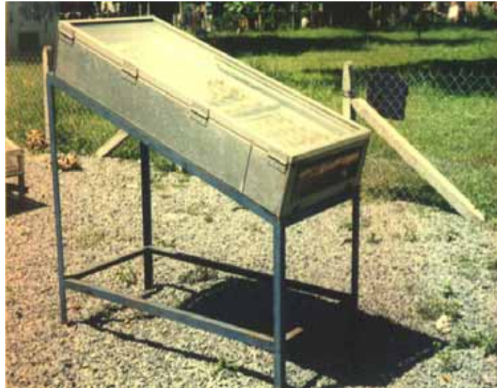
Figure 11.3: Fully assembled box type solar dryer
