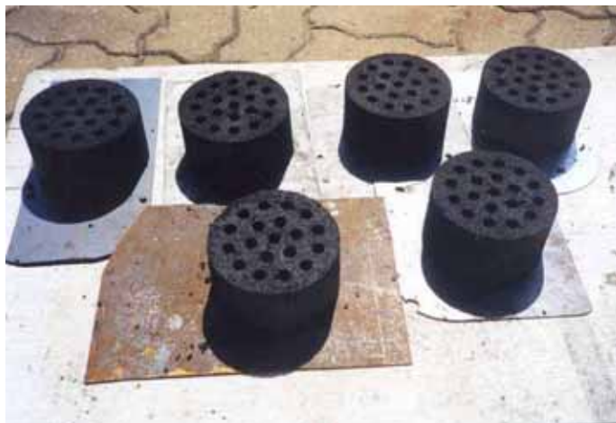
Figure 7.7: Drying of molded honeycomb briquettes
