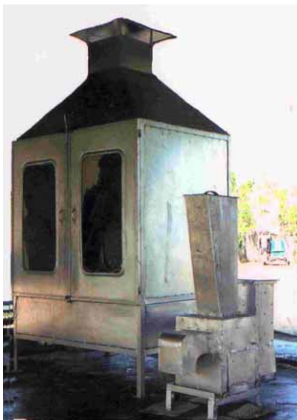
Figure 8.1: Drying chamber and biomass stove of the FD-50 Dryer
