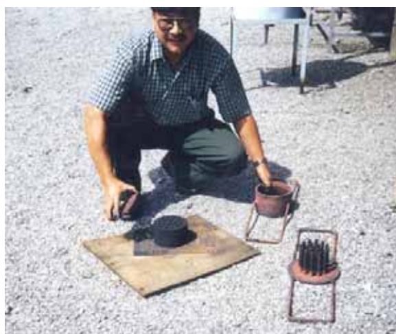
Figure 7.6: Briquette-making using the mould
