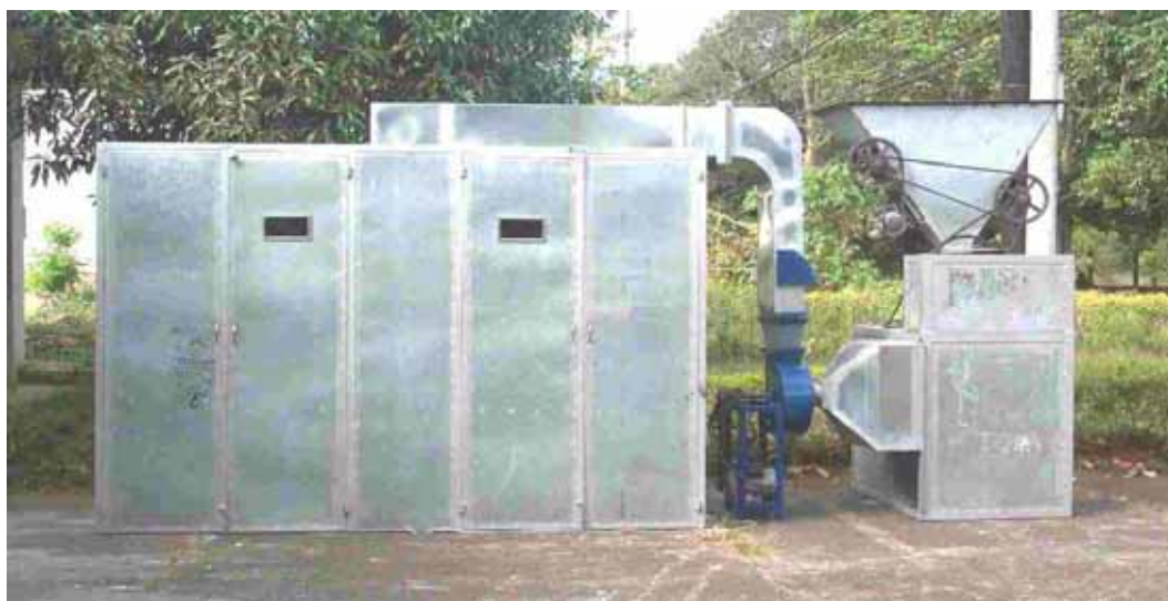
Figure 9.1: The rice husk-fuelled cabinet dryer FD-200
