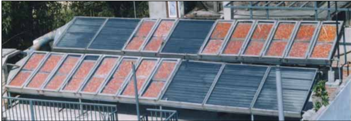
Figure 6.1: Improved solar tunnel dryer (split into two parts and connected using a U-connector)
