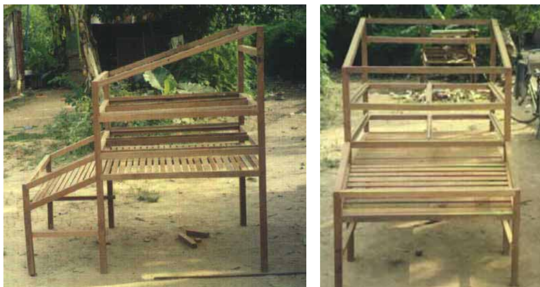
Figure 12.2: Base frame of solar cabinet dryer – 1 m 2 model
