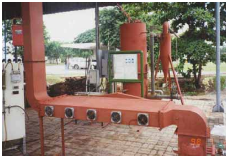
Figure 3.3: Biomass stove-heat exchanger unit without insulation
