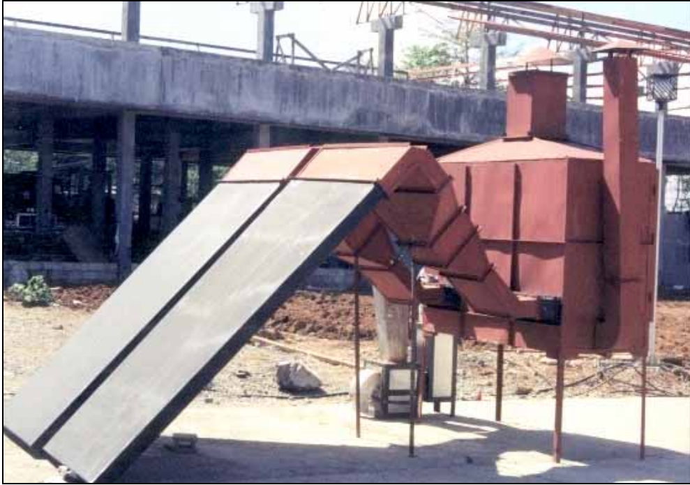
Figure 10.4: The transpired collector solar-biomass hybrid cabinet dryer
