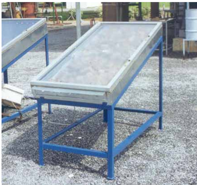
Figure 1.1: A fully assembled direct-solar box dryer
