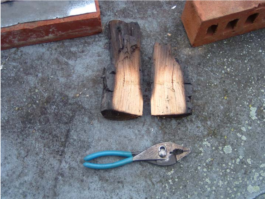
Figure 6: Large piece of wood that was partially pyrolyzed.
