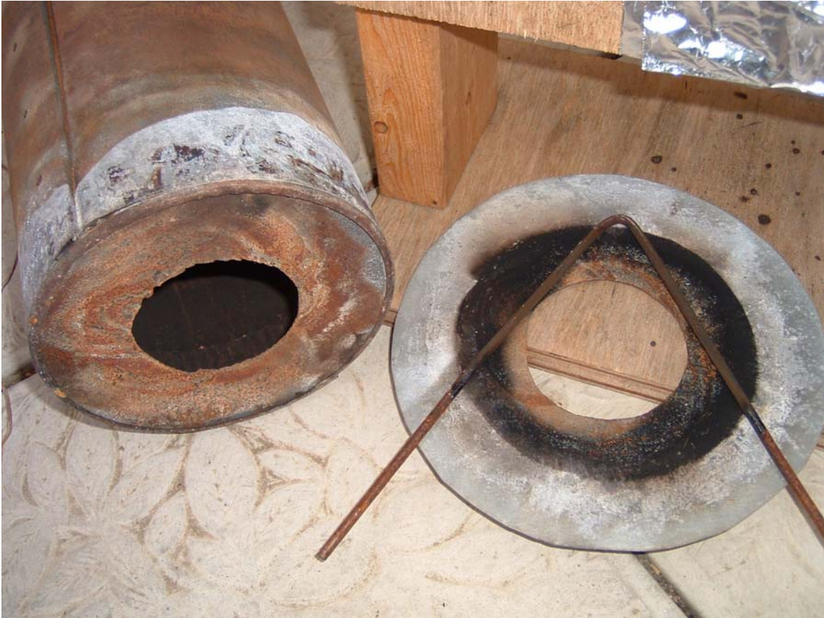
Figure 5: Two forms of the concentrating plate. On the left is a single piece built into the bottom of the riser. On the right is the concentrating plate as a separate piece, with the spacer wire shown as well. The bottom center of the plate is sooty.
