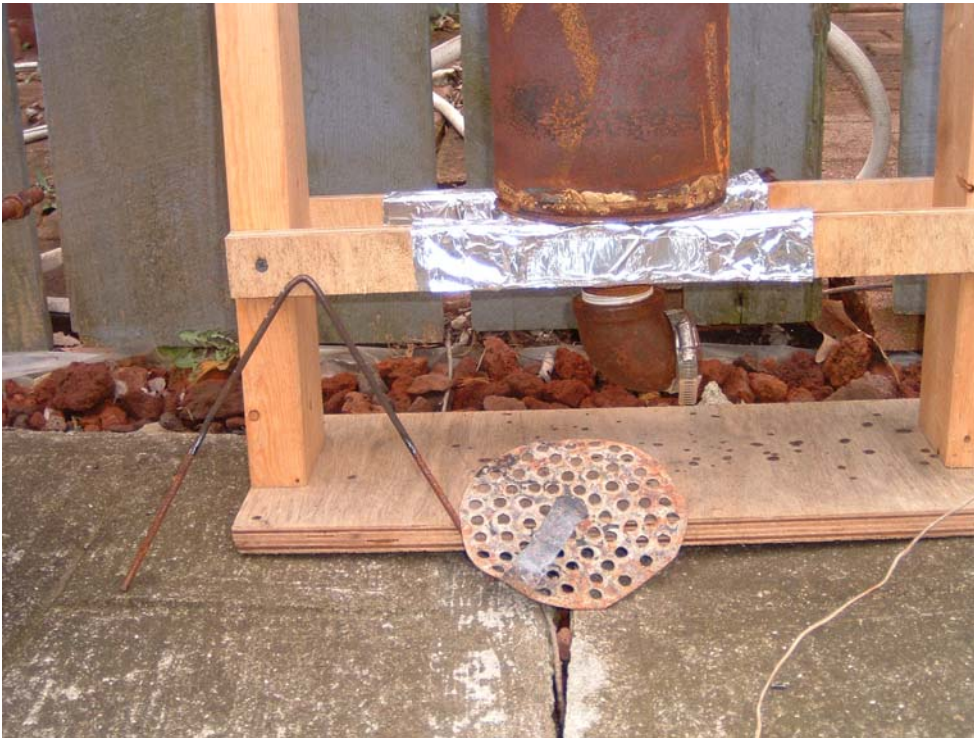
Figure 3: Base of the stove showing the air inlet. The grate and spacer wire are shown removed from the stove.
