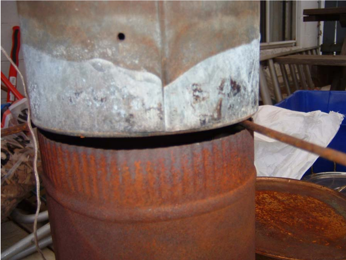
Figure 4: The ring-shaped gap which allow secondary air to enter the stove. The width of the gap is the diameter of the wire, which in this stove was 3/16 inch.
