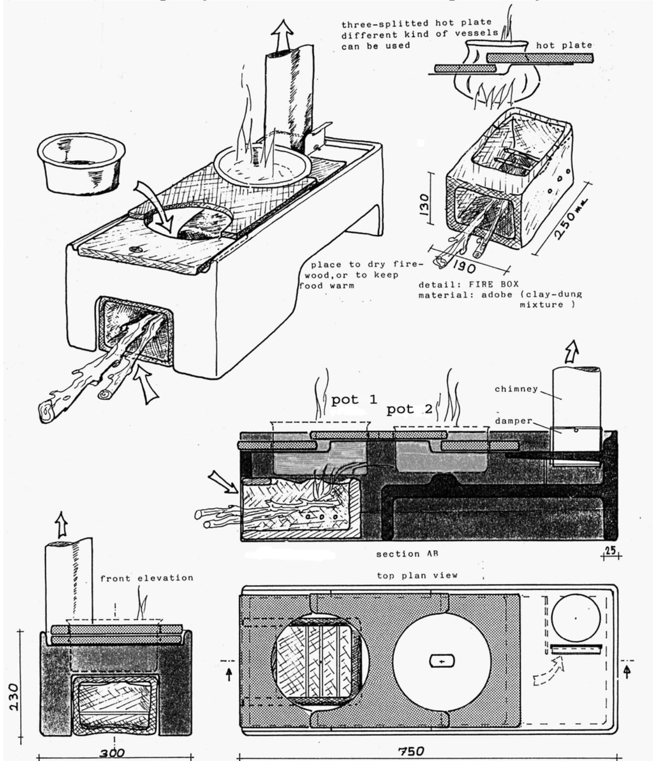
**CONCEPT:** This low-mass cooking stove achieves more than 30% fuel saving, compared to a three stone open fire, because the heated surface of the cooking pots is larger than the part of the pots which is cooled by the surrounding air. Both cooking pots are sunk inside the stove plate.
