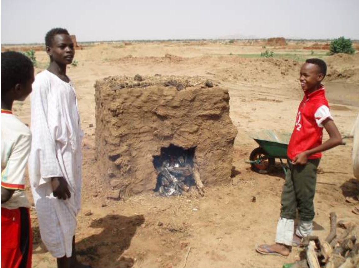
The test bricks are burned in this mini-kiln.
