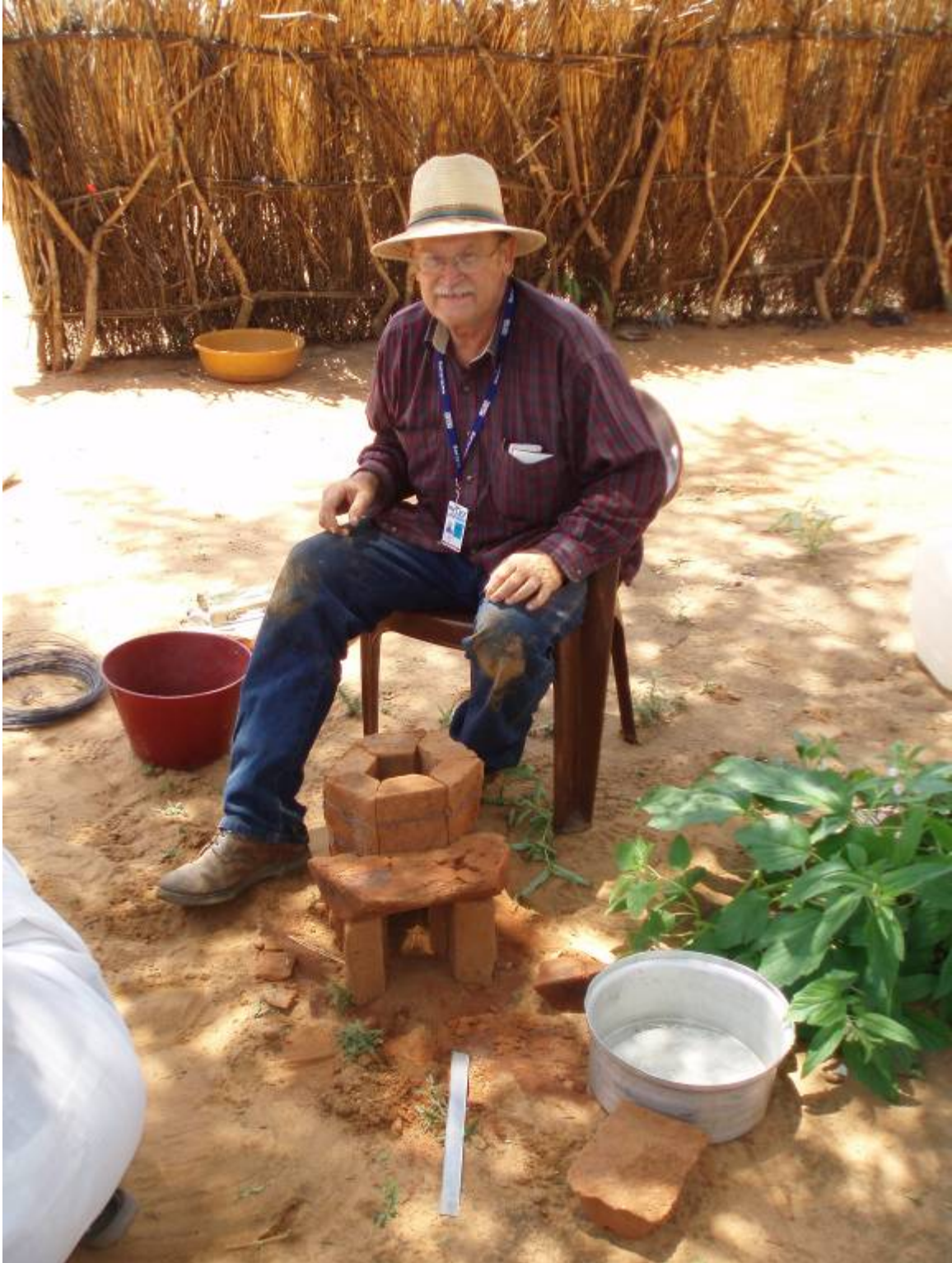
The Six Bricks Rocket Stove should actually be called the eight bricks rocket stove. While six bricks form the combustion chamber, two more bricks are used for the wood entrance or "elbow". (Wood ashes will insulate the bottom of the stove).
