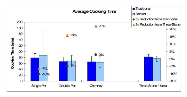
Differences in cooking times between the Rocket stoves and the traditional stoves were generally negligible. The double-pot stoves saved about 20% of the time as compared to the single pots (including three-stone and kerosene). The chimney stove required the same average amount of time as the non-chimney double pot to cook the meal. The single pot Rocket stove was slightly slower to cook compared to the open fire but the two pot stoves were 16% and 22% faster.
