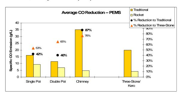
The reduction in carbon monoxide of the stoves is of a similar magnitude to the PM reduction. Again, Kerosene did emit fairly high levels of CO. The CO emissions seemed to be more of a steady-state artifact of kerosene combustion rather than due to start-up and cleaning of the stove.
