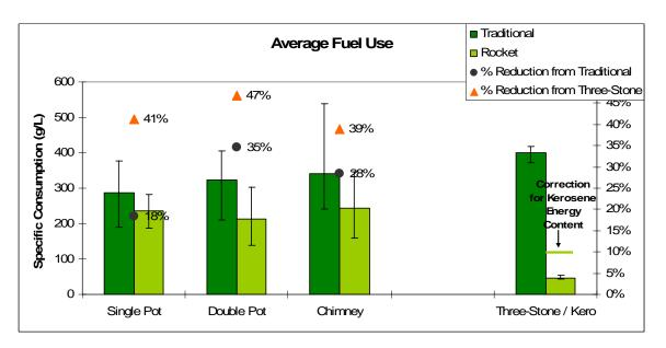
The single pot Rocket stove (without pot skirt) used 18% less fuel compared to the traditional stove. It saved 41% of the fuel compared to the open fire. The two pot used 35% less fuel compared to the traditional stove and saved 47% compared to the open fire. The chimney stove followed the same pattern by reducing fuel use by 28% compared to the traditional stove and 39% compared to the open fire.
