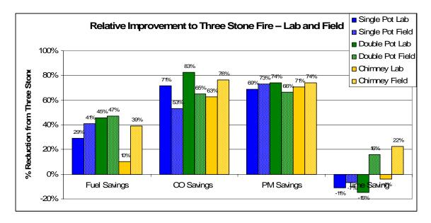
Generally there was a good agreement when comparing the total emissions from the stoves to the three stone as measured in both the lab and field. Fuel savings was greater in the field, anywhere from 2% in the two-pot to 29% with the chimney stove. Reduction in CO was less than expected in the field from the non-chimney stoves with an 18% difference. There was a13% improvement from the chimney stove in the field.
