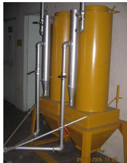
The Dual Reactor Rice Husk Gasifiers with Gas-Pipe Burner
