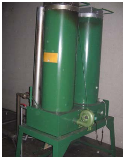
The Dual Reactor Rice Husk Gasifiers with Gas-Pipe Burner
