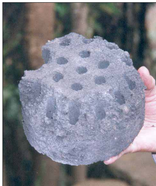
Poor quality briquettes disintegrate during transport.
