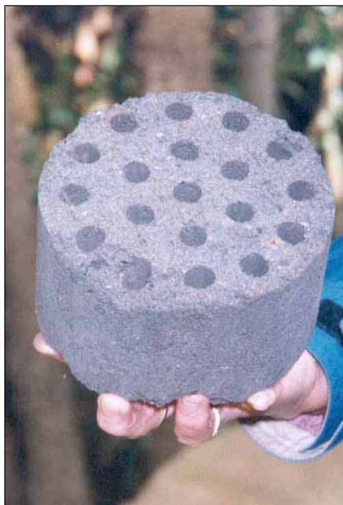
Poor quality briquettes disintegrate during transport.
