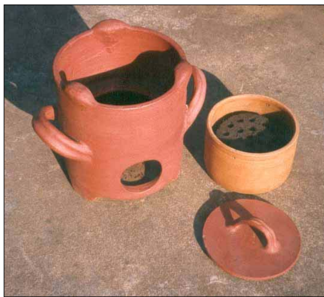
Briquette Stove from which the insulations has been removed (left) and Baked Clay Stove (Right)
